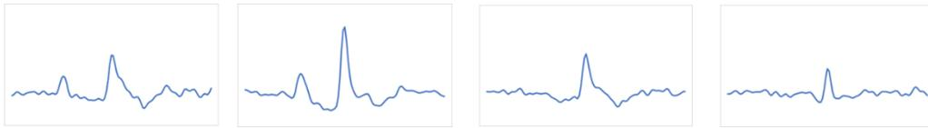
a) Typical waveforms after filtering and spike detection
