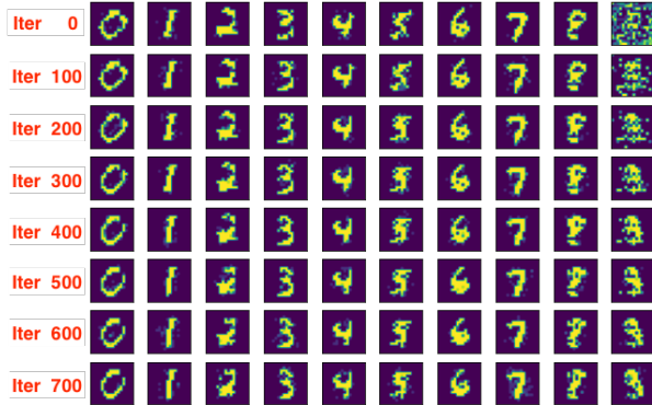
Figure 10: Online Incremental Learning: STDP learns a previously unseen input number '9' within 500 examples.
