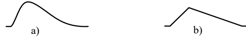
Figure 2. Two response functions. a) Biologically-based biexponential response function that is the difference of two exponential decays. The faster decay models the decrease in synaptic conductance that follows the sudden increase caused by an input spike; the slower decay models membrane leakage. b) Piecewise linear approximation of biexponential response studied by Maass [32].
